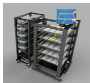
Schematics of a DTP which consists of 120 microfluidic devices, and a photo of an example of a microfluidic device. The details of the system and the device are described in the research description.
