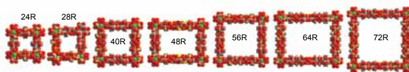
Figure 1. Systematic expansion of structures with extra-large channels with ring size ranging from 24R to 72R.
