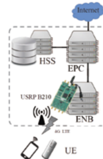
Fig. 1. Architecture of a real testbed for software RANs.
