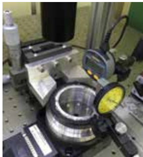
Fig. 1: Integration of rotary-magnetic encoder on direct drive motor.
