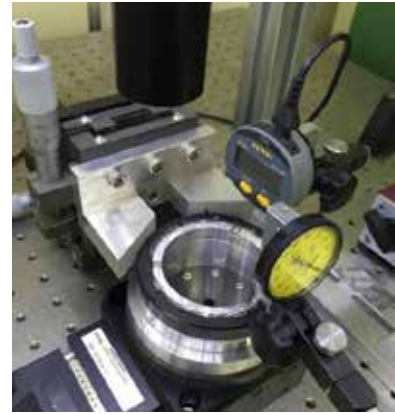
Figure 1. Integration of rotary-magnetic encoder on direct drive motor.
