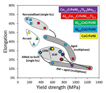
The yield strength (1235 MPa) and ultimate tensile strength (1550 MPa) achieved in this work are the highest to-date for HEAs subjected to laser additive manufacturing processes.
