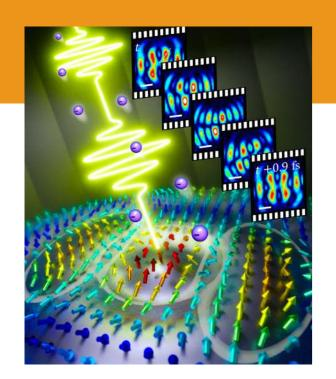
An interferometric photoemission electron microscope is used to time-resolve the vectorial surface plasmon vortex fields and reveal the corresponding spin textures.
