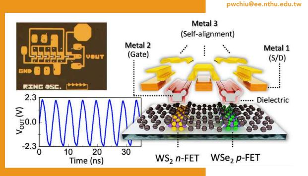
Schematic illustration of 2D FET architecture and measurement property of a ring oscillator thus made
